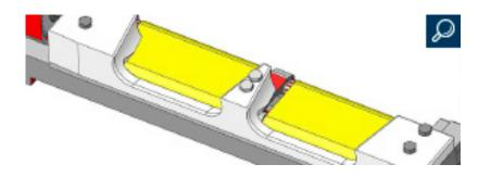
The powered slicing bar provides dynamic support to the product directly in front of the slicing bar on the slicer. The synchronised guides ensure product motion is perfectly controlled and guarantee that even elastic loaves of product are precisely conveyed.
